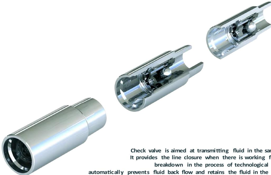
Check valve is aimed at transmitting fluid in the same direction. It provides the line closure when there is working fluid pressure breakdown in the process of technological operations, automatically prevents fluid back flow and retains the fluid in the tubing string.
